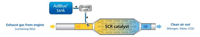
AdBlue® is a high purity solution of Urea, a synthetically produced chemical that is not hazardous to handle or transport.
